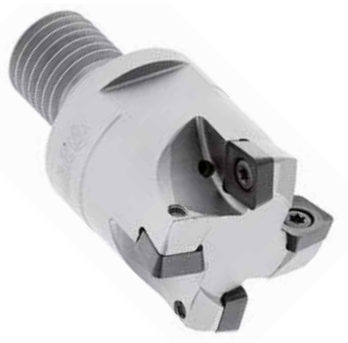
Threaded Coupling K r =10° | γ p =+2° | γ f =+2° | R p =0.079
