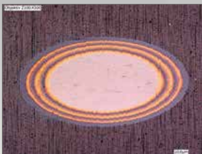
Calotte grind in a multi-layer coating
