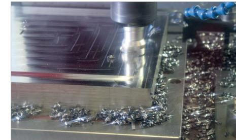
Workpiece material: 1.2738 Steel (34 HRC)
